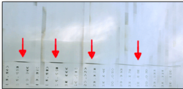
Figure 7: Misaligned pitch measurement printout (broken black lines)
